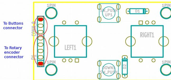
It connects to two connectors on the main board – 'Rotary encoders connector' and 'Buttons connector' (pin 4 of this connector is not used).
