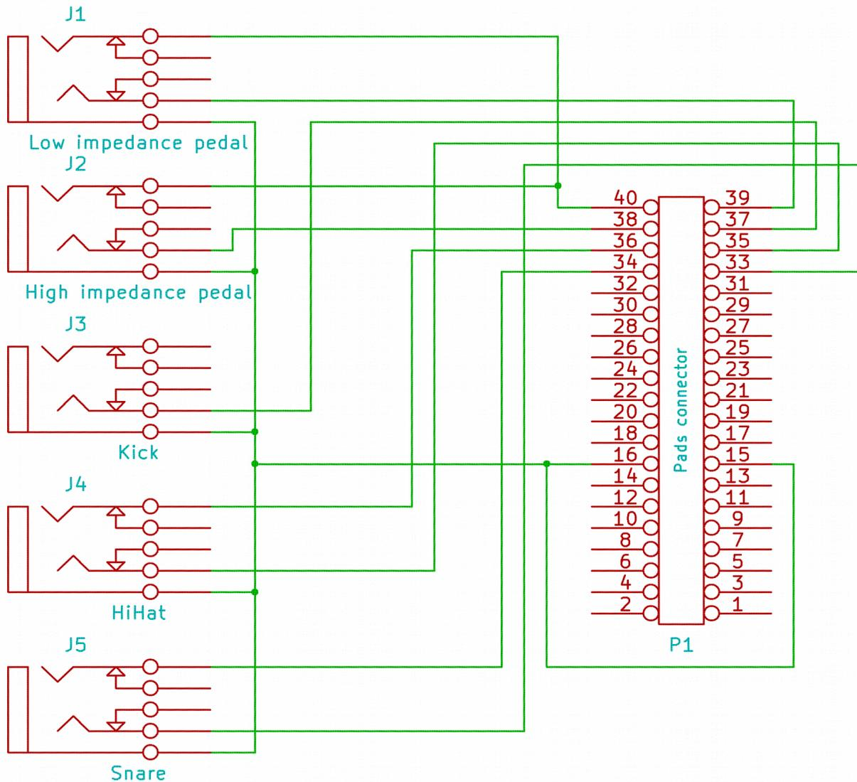
The rest of input jacks are wired to Pads connector 1 and Pads connector 2 as exemplified above using Pads connector pinout.
